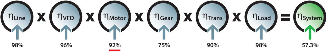
You can see in both examples that you are wasting over 45% of the energy going into the system. You can also see that replacing your motor with a premium-efficient model will save you less than 4 percentage points of efficiency. The other, less efficient components in your drivetrain are still wasting energy, meaning that the investment you've made in a premium-efficient motor will take longer to recoup than you had planned.
