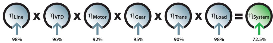
You'll see now we are quickly recognizing substantial, double-digit efficiency gains – nearly 20 percentage points – and your line begins to become much more efficient. If you change your transmission elements from a v-belt to a positive engagement method, or even to a direct-drive method, your efficiency gains can be even higher.
